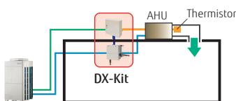
When connecting to an air handling unit, the supply air temperature is controlled by the discharge sensor.
