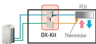
When connecting to a fan coil unit, the room temperature is controlled by the return air temperature sensor.
